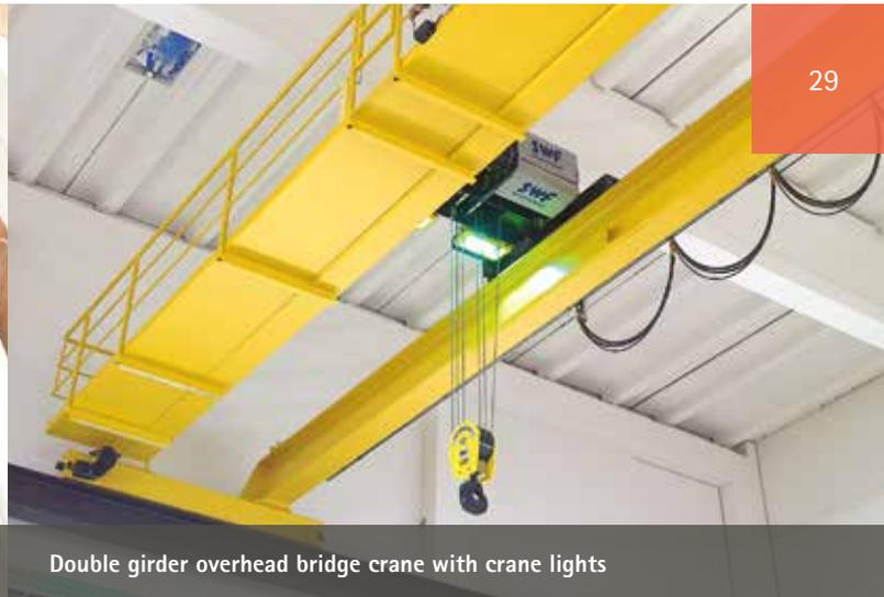
Double girder overhead bridge crane with crane lights
