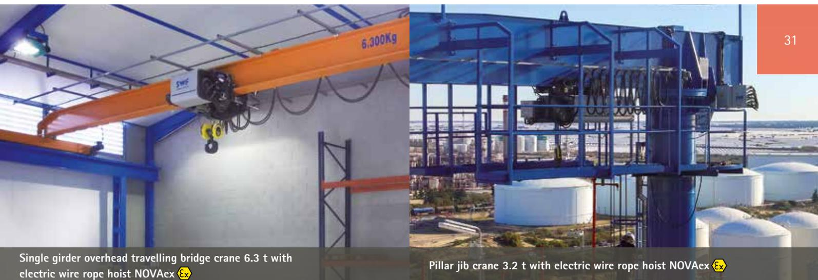
Single girder overhead travelling bridge crane 6.3 t with electric wire rope hoist NOVAex
